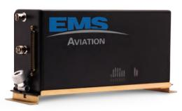
The Sky Connect Iridium® transceiver enables global voice, text, tracking and data communications with the Iridium satellite network.
